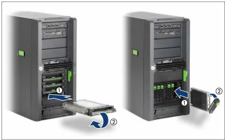
Figure 26: Installing the 3.5-inch and 2.5-inch HDD modules
